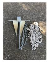
12 lb. Danforth anchor with 5.5 feet of chain (6 lb.) and 145 feet of rope rode marked at 30, 60, 90, and 120 feet above the anchor. \$90
